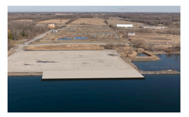
The project aims to improve the existing facilities by installing a 104m section of sheet pile to create a new wharf face in between two existing dock structures known as dolphins. These improvements will create a safe and stable platform to make it easier to load and unload different types of cargoes and accommodate a wider variety of vessel types.
